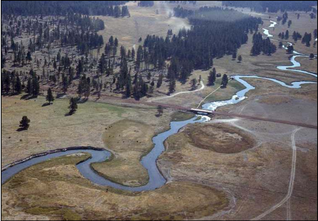
Photo 8-7. View of Upper Williamson River at Rocky Ford Channel incision is more pronounced downstream (left side of picture) of the bridge.
